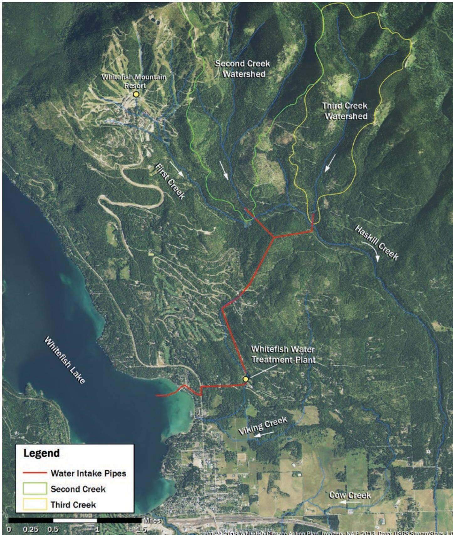
FIGURE 2. MAP OF HASKILL BASIN AND CITY WATER INFRASTRUCTURE. Two tributaries to Haskill Creek provide most of the City’s drinking water, supplemented by water pumped from Whitefish Lake during periods of low flow and peak demand.
