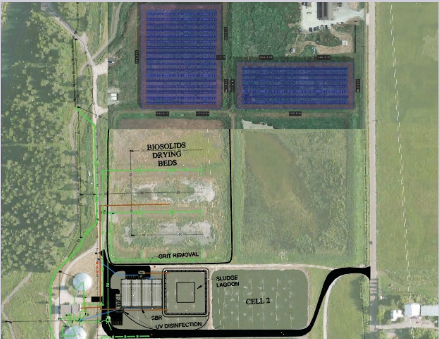
FIGURE 4. PRELIMINARY SITE DESIGN OF NEW WHITEFISH WASTEWATER TREATMENT PLANT. Showing proposed 1.7 MW solar farm (blue). Courtesy Anderson-Montgomery Consulting Engineers and Aeon Renewable Energy.
